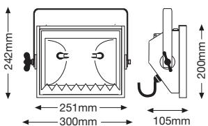
Stylish and high specification 500W asymmetrical floodlights, ideal for professional usage in all cyclorama-type lighting applications. Rima A500F is designed for usage as single module flood, but a large choice of different models and accessories is available for the creation of multiple rows or square-battens. Rima A500 is delivered complete with colour frame and 1.5m mains cable.
