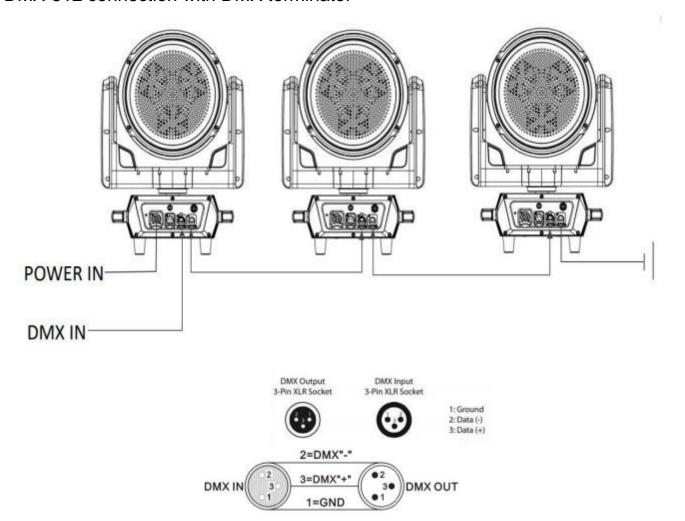
For installations where the DMX cable has to run a long distance or is in an electrically noisy environment, such as in a discotheque, it is recommended to use a DMX terminator. This helps in preventing corruption of the digital control signal by electrical noise. The DMX terminator is simply an XLR plug with a 120  $\Omega$  resistor
