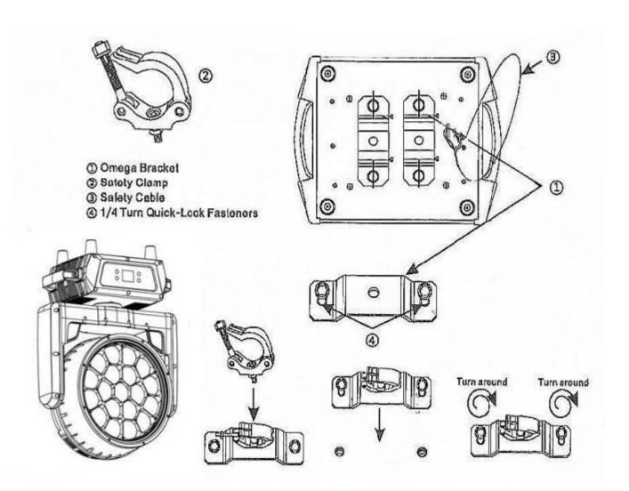
Regardless of the rigging option you choose for our fixture, always be sure to secure your fixture with a safety cable. The fixture provides a built-in rigging point for a safety cable on the hanging bracket as illustrated above. Be sure to only use the designated rigging point for the safety cable and never secure a safety cable to a carrying handle.
