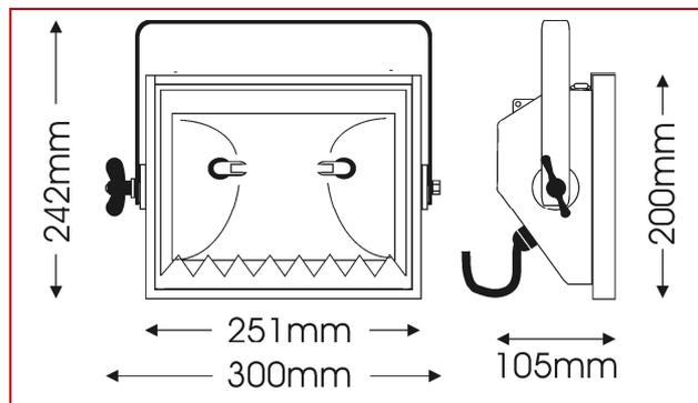
New, stylish and high specification 500W asymmetric floodlights, ideal for professional usage in all cyclorama-type lighting applications.
