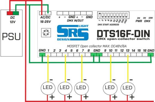
There is a 12V power supply with the output used for load connection of LED strips and DTS16-F DIN, on the picture. The "+" pole of the strip must be connected to the power supply and the "-" one to the DTS16F-DIN switching channel.
