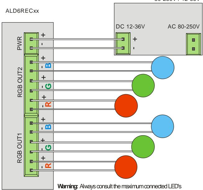
Always calculate the apropiate PWR power supply depending on the LED fixture used. If you need help just ask at tech@srslight.com. That should avoid a lot's of problem and burned fixtures!!!
