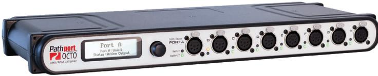
The Pathport OCTO operates on wall power, accepting an input voltage between 100-240VAC at either 50 or 60 Hz. The AC outlet shall be near the equipment and shall be easily accessible. There is no on/off switch. This equipment relies on building installation overcurrent protection.
