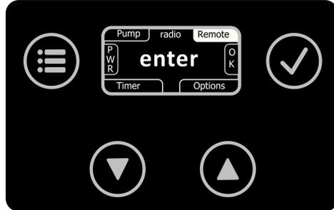
Up to 60 different handheld transmitters can be programmed on the machine. For this purpose, the "Remote" submenu must first be selected.
