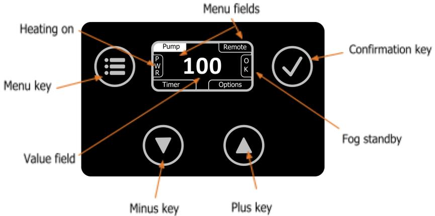
The Classic<sup>2</sup>/Highpower<sup>2</sup> is operated via the four keys (menu, minus, plus, confirmation) and the OLED display. The menu fields are located in the corners of the display, and the value field, which displays the value of the selected menu field, is located in the center. The menu key is used to select the individual menus counterclockwise. The corresponding value can then be changed with the help of the plus and minus keys and then saved with the confirmation key.
