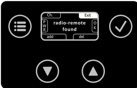
In the Remote submenu, the menu fields are replaced. The channel (key on the handheld transmitter) can be selected at the top left. At the bottom left, a new hand-held transmitter is taught-in and at the bottom right, the taught-in hand-held transmitters are deleted again.
