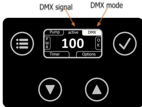
If a valid DMX signal is present, this is displayed at the top center with "active". The currently read pump value can be displayed by selecting the pump menu item. If the received value is greater than zero, the Classic<sup>2</sup>/Highpower<sup>2</sup> starts the fogging process and stops it accordingly at the value zero.
