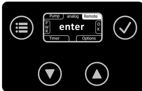
After plugging in the cable remote control, the Classic<sup>2</sup>/Highpower<sup>2</sup> automatically recognizes that an analog cable remote control has been plugged in. On the cable remote control there is an on switch and a potentiometer for setting the pump value.
