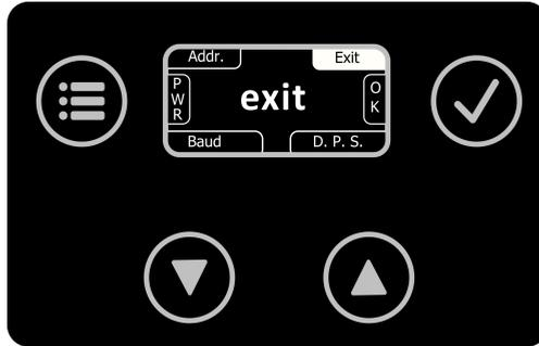
In the Modbus submenu the menu fields are replaced. At the top left the address of the device can be set. At the bottom left the baud rate of the communication is set and at the bottom right the data width, parity and stop bits. The setting is done analog to the main menu.
