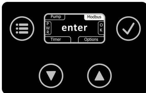
The communication parameters of the connection can be set in the "Modbus" submenu. First, the Modbus menu item must be selected. Enter" is displayed in the value field. The confirmation key is used to access the submenu for Modbus.
