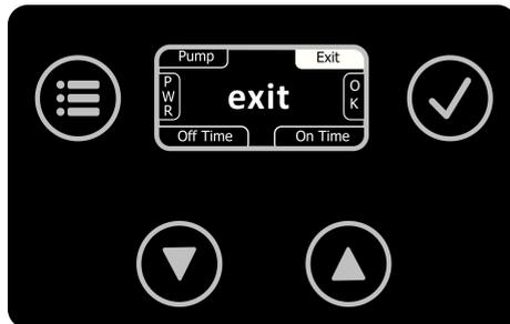
the waiting time can be set in 0.1 minute ( 6 sec.) steps. Analogously, the fogging time can be set in steps of seconds at the bottom right.
